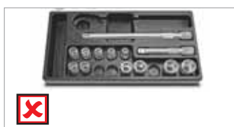
Better organization but no indication of missing tools.
