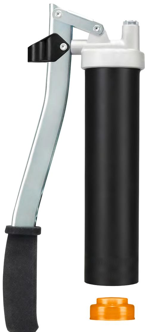
The new easyFILL 400 works without the need of any spring mechanism. Simply insert the cartridge, insert the follower plate and get started. The vacuum in the grease gun head moves the piston smoothly upwards all by itself. Through the Variable Stroke principle the grease gun can be easily operated with minimal lever movement.
